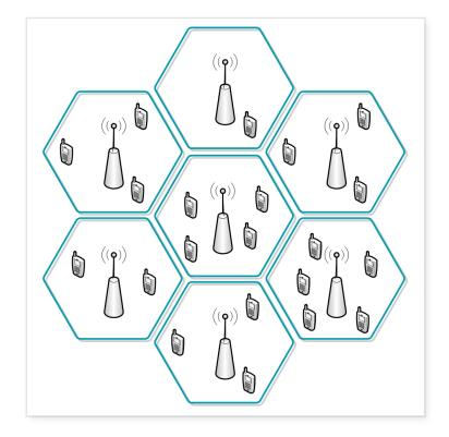
Until recently most mobile networks were made up of cells which covered a range of about half a mile to five miles from the tower. These big cells that are served by big towers, and big antenna, are called *macro cells*.
