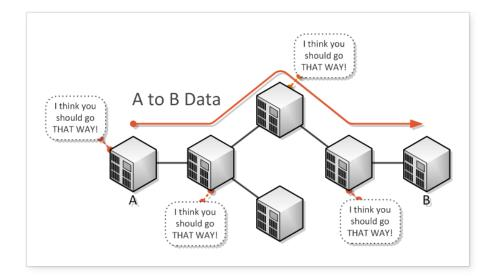
This autonomy was one of the great benefits of IP networks as it meant that the network itself could react to reconfiguration and faults extremely quickly, without needing an engineer to intervene.
