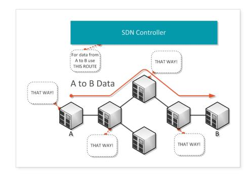
Traffic routing is not all that SDN improves. SDN is also a movement away from proprietary management tools to open API standards. A lot of the IP hardware vendors' work went in to implementing and maintaining protocols in their routers and switches, and that drives up the cost of traditional devices.
